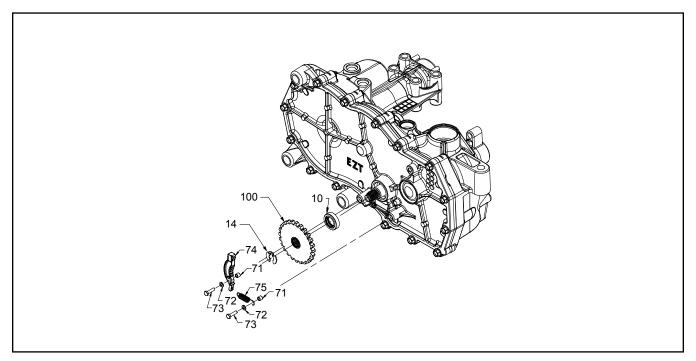
Figure 8. Cog Brake Assembly
