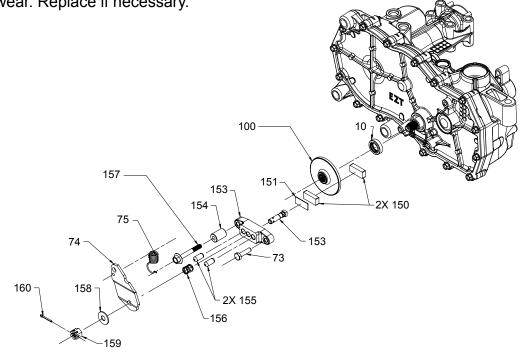
Figure 9. Disc Brake Assembly
