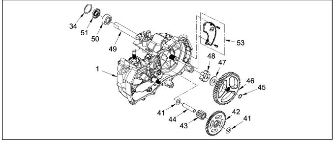
Figure 11. Axle Shaft, Reduction Gears and Expansion Plate
