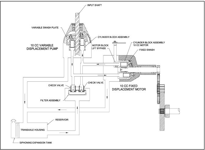
Figure 2. Hydraulic Flow Illustration
