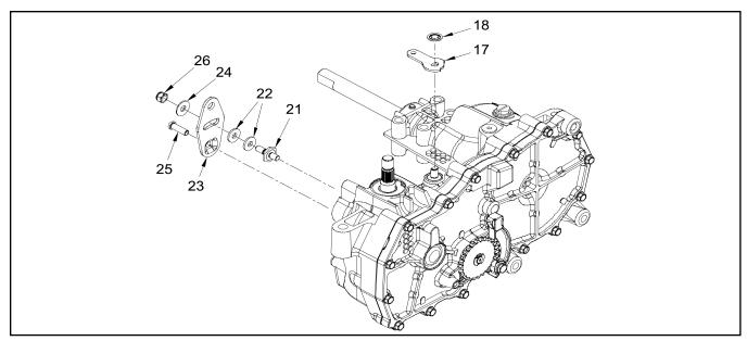
Figure 6. Control Arm and Bypass Arm
