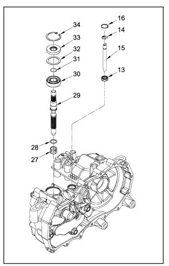
Figure 13. Input Shaft and Bypass Rod Assembly
