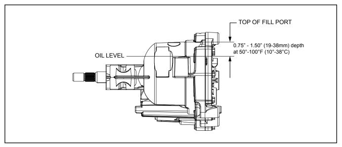
Figure 4. Fluid Level and Fill Port
